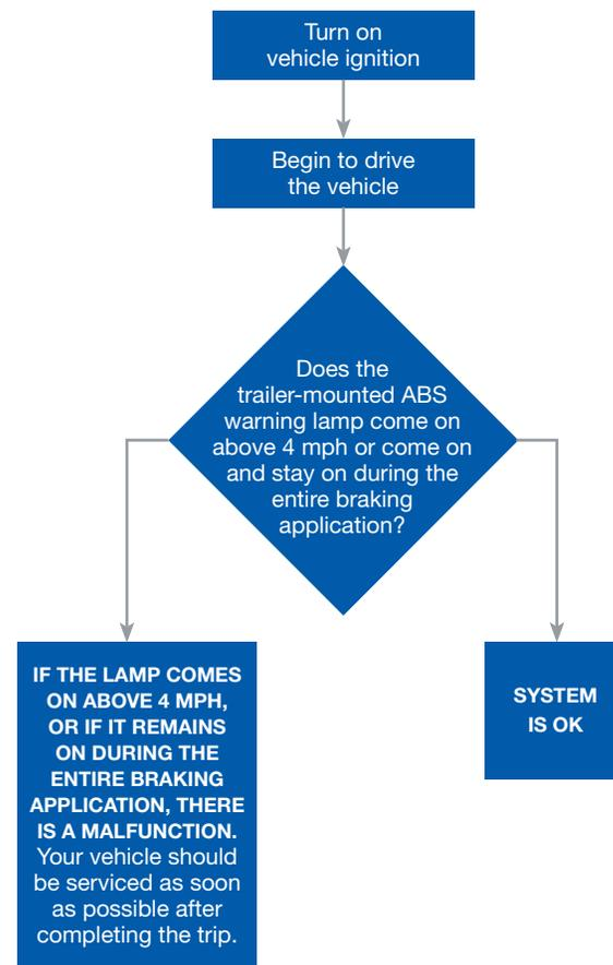
**Note:** Depending how the ABS is powered, the lamp may come on briefly at ignition and then go off, or briefly flash each time you apply the brakes on a moving vehicle.
